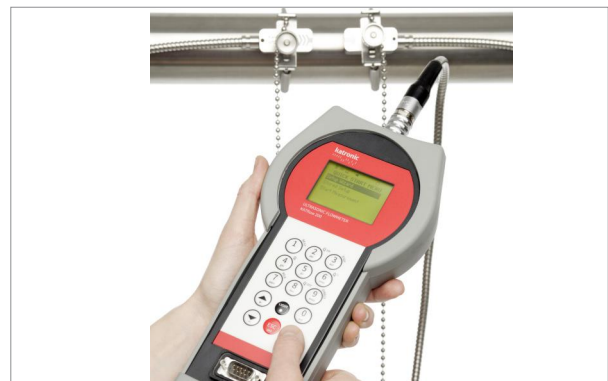
KATflow 200 in operation
