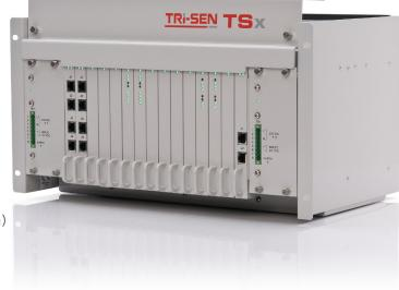
Turbomachinery applications require a number of special types of I/O, such as pulse counters, LVDT interface, temperature inputs and various voltage interfaces. The TSx is able to interface with these I/O functions directly, eliminating interposing transducers that can create a single point of failure in some of the most important I/O loops of the control system.
