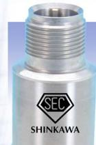
**The HS-100I and HS-100SI Series** of industrial accelerometers are AC versions which are ATEX and IEC Ex certified for use in Group I and Group II potentially explosive environments. They typically operate over a temperature range of -67 to 284°F (-55 to 140°C) and cover a frequency response over 2 Hz to 10 kHz.
