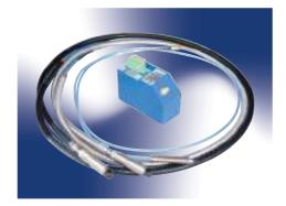
The FK-202F transducer is the eddy current type non-contact displacement/vibration transducer, used for measuring Shaft Vibration, Axial Position, Rotating Speed and Phase Mark (Phase Reference) from small rotating machinery to large critical machinery such as turbines and compressors in plants.
